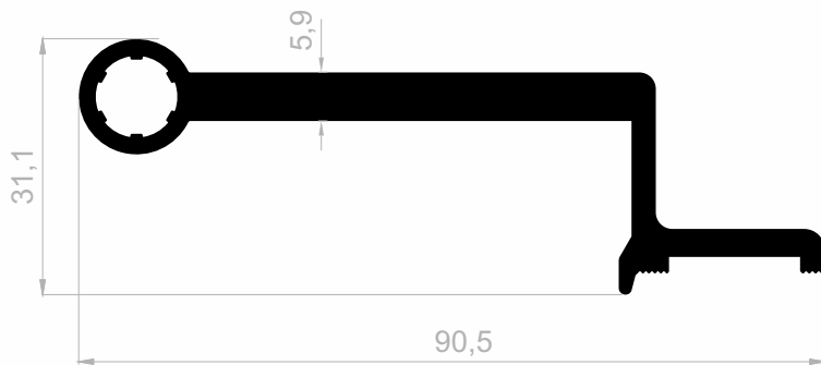
J 1621 HINGE PROFILES WEIGHT : 1,499 kg/m
