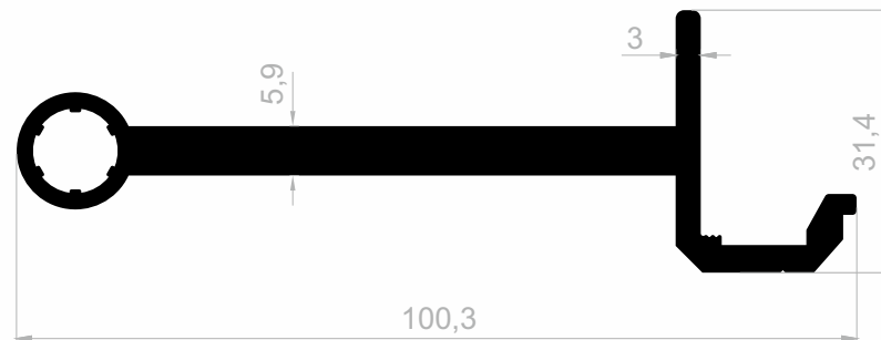
J 1619 HINGE PROFILES WEIGHT : 1,696 kg/m
